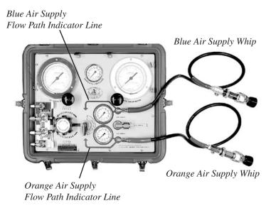
Fig. 3 Air flow paths from the H.P. cylinders.
